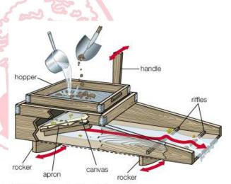
hopes of extracting gold from the bottom of the pan. 93 While this method was simple and cost-effective, it was not efficient. Another method of gold extraction was by rocker box. A rocker box works similarly to the panning method but on a larger scale. A prospector would place dirt from a creekbed in the top hopper, pour water on the soil in the hopper, and then rock
